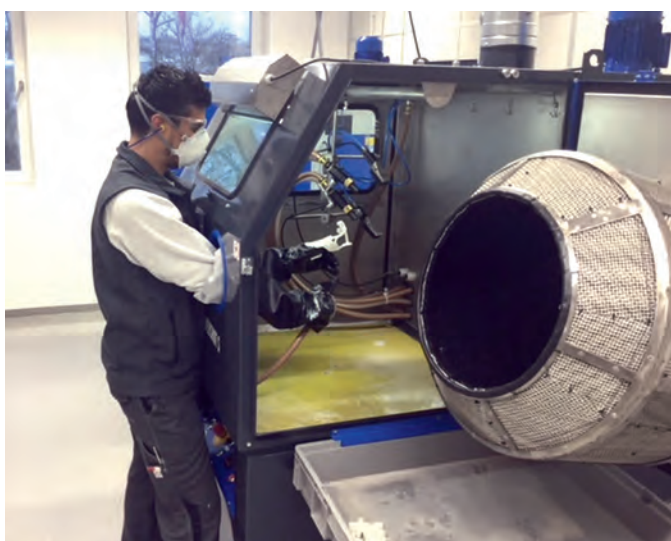
Fig. 14 Final surface finishing before the colouring process.
