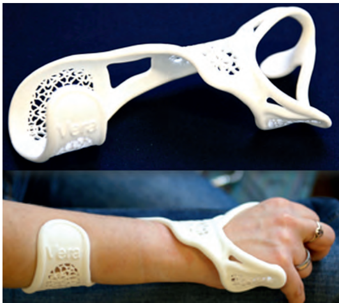
Fig. 12 Ready-to-try 3D printed workpiece made of polyamide after the printing process.
