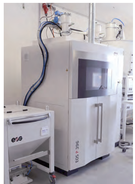
Fig. 11 EOS SLS printer for producing customised orthopaedic devices.
