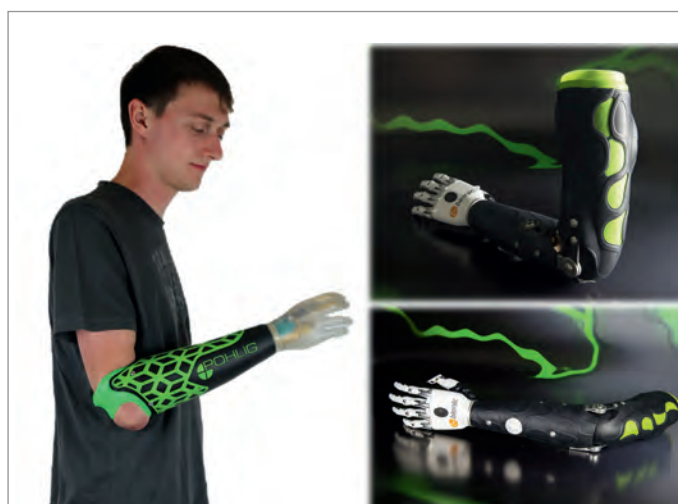
Fig. 15 Pohlig 3D printing design studies on upper limb prosthetics.
